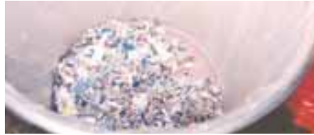
WASTE PLASTIC SHREDDED INTO CHIPS
