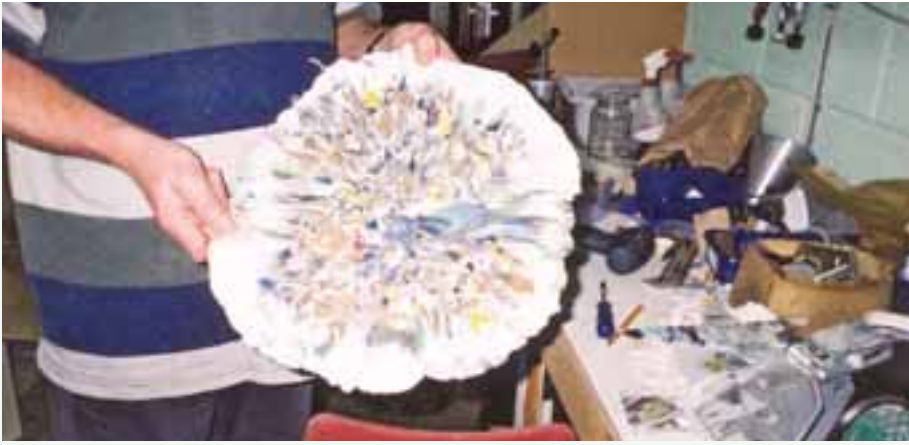
WASTE PLASTIC PRESSED IN A HYDRAULIC PRESS, READY TO BE CUT INTO SHAPES
